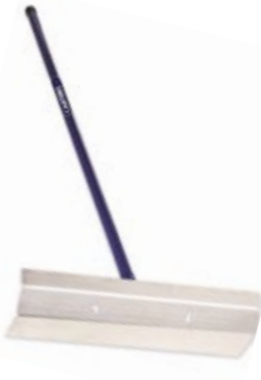
CPLAALS Aluminium Concrete Placer Handle: Tubular Steel Blade: 508 x 152mm Handle length: 1500mm Weight: 1.5kg
