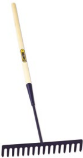
16AREP 16T Sq. Asphalt Rake Handle: Hardwood Blade: 406 x 102mm Handle length: 1680mm Weight: 2.5kg
