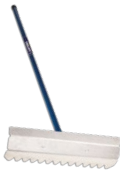
CPRAALS Aluminium Concrete Rake Handle: Tubular Steel Blade: 508 x 152mm Handle length: 1500mm Weight: 1.5kg
