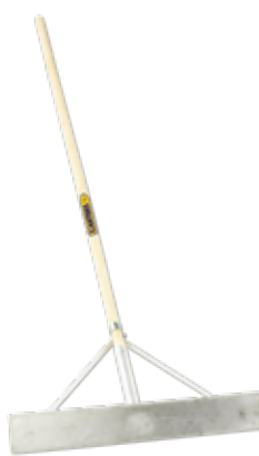
ALUSPA Aluminium Spazzle Handle: Hardwood Blade: 600 x 125mm Handle length: 1500mm Weight: 1.7kg
